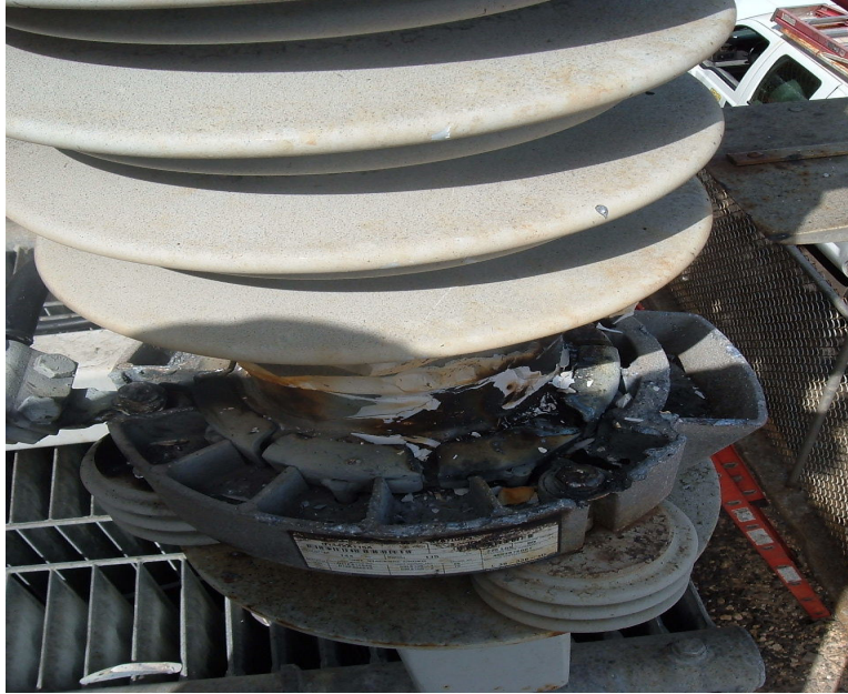
Photo #2: Burnt outer phase arrester base
